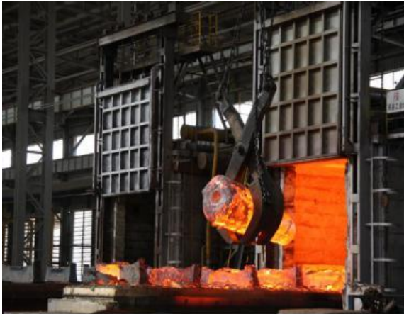
Forging heat furnace
